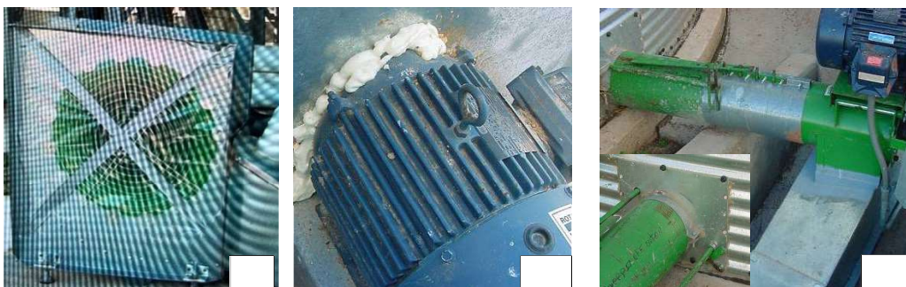
Fig. 5. Sealed fan inlet with plastic and X-braced (A), fan motor shaft foam sealed (B), caulk auger push rods and foam inside tube (C).
