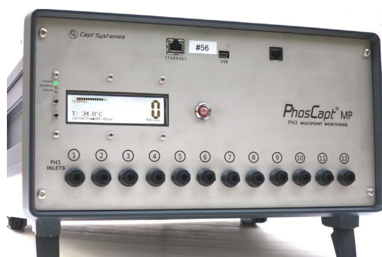
Fig. 1. PhosCapt®-MP: 12 lines Phosphine monitor. CaptSystemes, France. (phoscapt.com)
