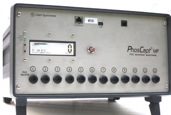
Fig. 1. PhosCapt®-MP: 12 lines Phosphine monitor. CaptSystemes, France. (phoscapt.com)
