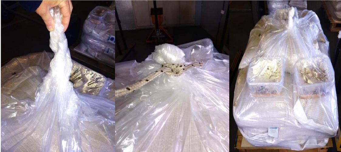
Fig. 1. Sealing method of the modified atmosphere chamber. Left: opening of the bag twisted; Center: close-up of knot sealing the modified atmosphere chamber; Right: detail of a sealed chamber with the oxygen scavenger inside.
