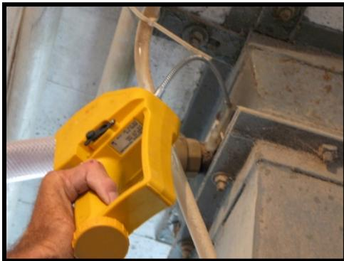
Fig. 4. Electronic gas monitor.
