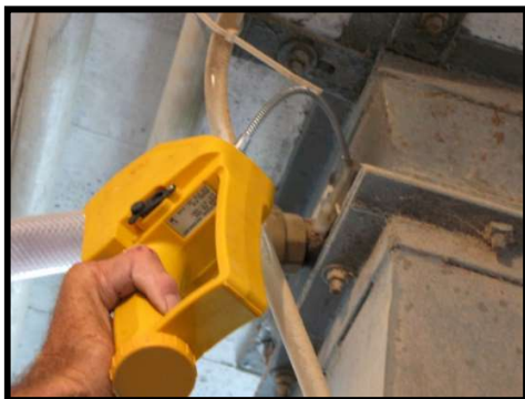
Fig. 4. Electronic gas monitor.
