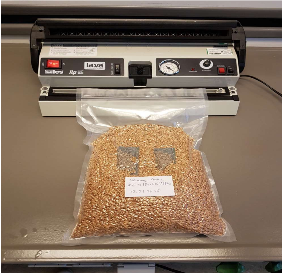
Fig. 1. Vacuum machine with welding station and vacuumized wheat bag with two nylon gauze cages containing 100 grains with immature stages.
