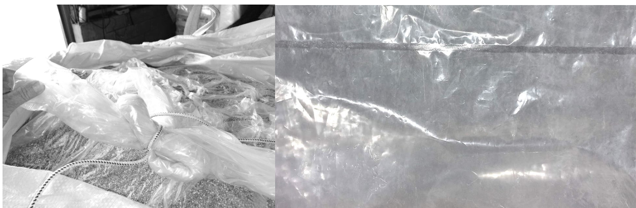
Fig. 1. Left: Big bag closed using the twisting-folding-knot system. Right: Big bag closed using the heat-sealing method (indicated by arrow).
