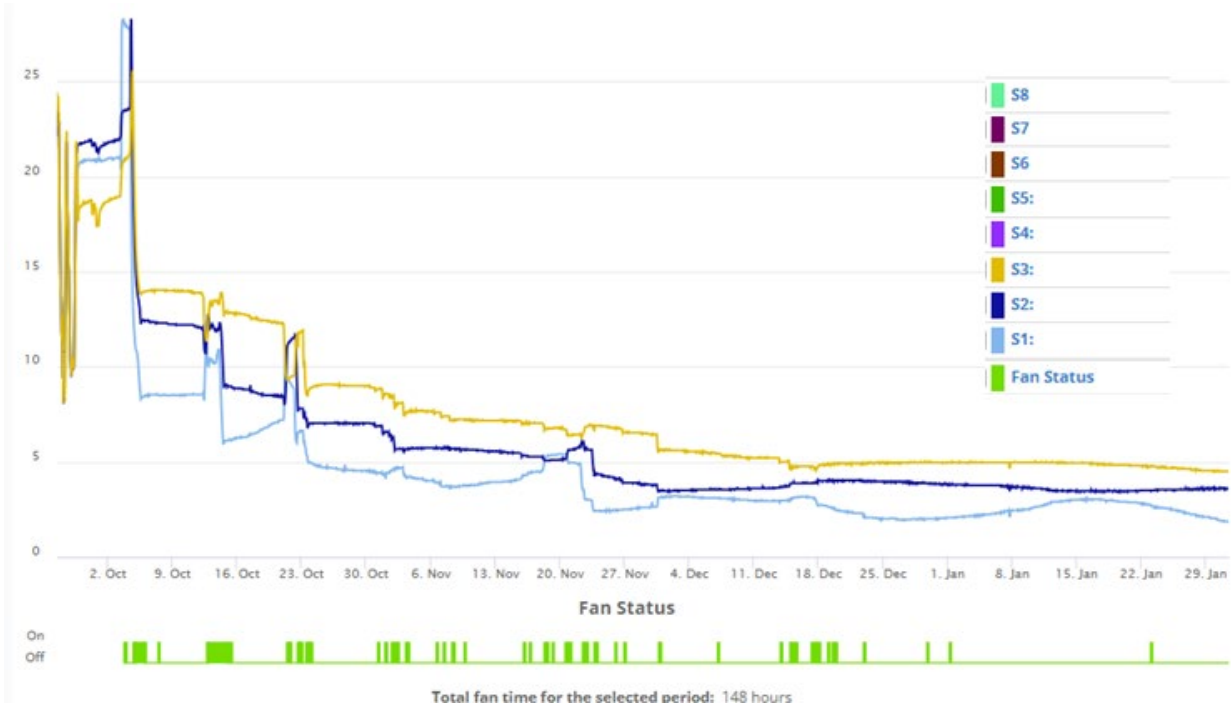
Fig. 1. Temperature (°C) profile of the bin with stored canola over the storage period.
