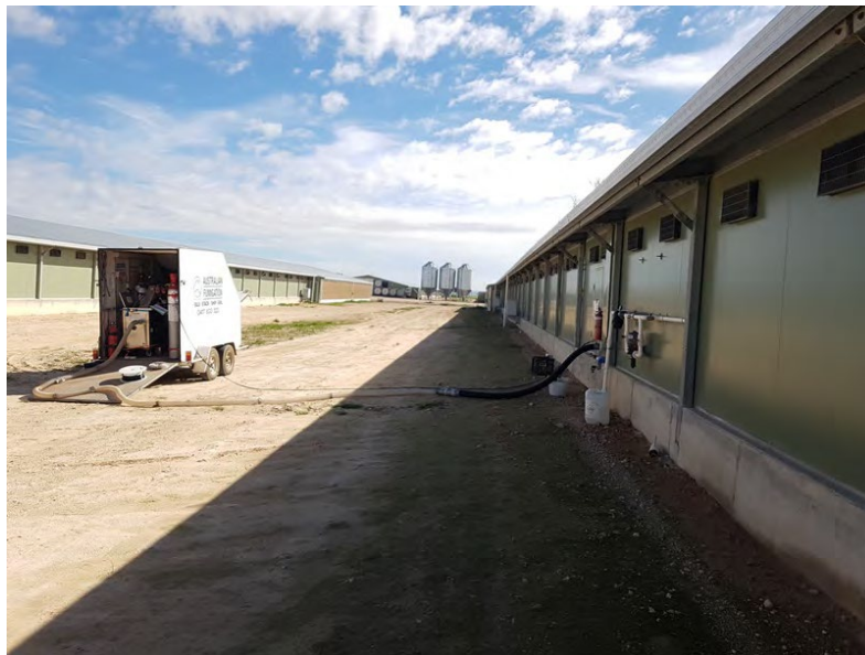
Fig. 2. Setup of the VAPORPH3OS ® cylinder and the HDS 200 phosphine/air mixer in a trailer and hose connection into the middle side of the poultry house.
